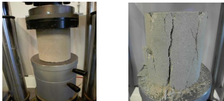
Figure 4.1 Monotonic compressive testing and specimen after failure
