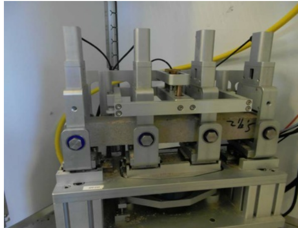
Figure 4.23 Four-point bending test setup
