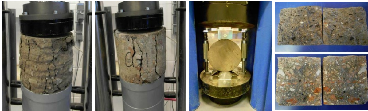
Figure 7.19 Compression and indirect tensile strength tests
