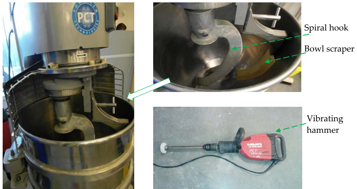
Figure 3.13 Mixing and compacting equipment
