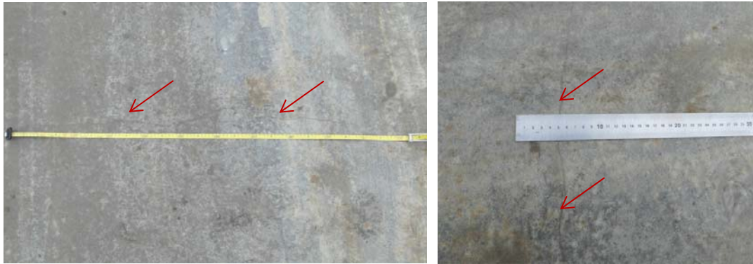
Figure 7.15 Observed cracks in stabilized sand section S-1
