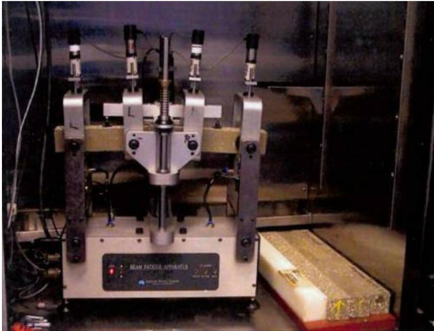
Figure 1. UTM 4 point bending test cell for fatigue measurement (with the test piece made with ImmoCem 35/0,3)
