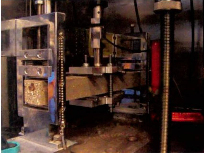
Figure 2. 4-points load cell equipment as used in the tests in UTM-elaboration (the test beam shown was produced with ImmoCem 35/0,3)
