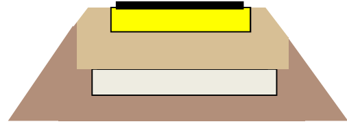
Figure 3.17: Remediation using the PowerCem technology
